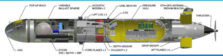
The Explorer class nupiri muka is a large modular AUV capable of operating in some of the most difficult conditions on earth, including beneath floating ice shelves. This vehicle has flexible payload options and can dive to 5000m and travel at speed between 1.0-2.5 m/s.
