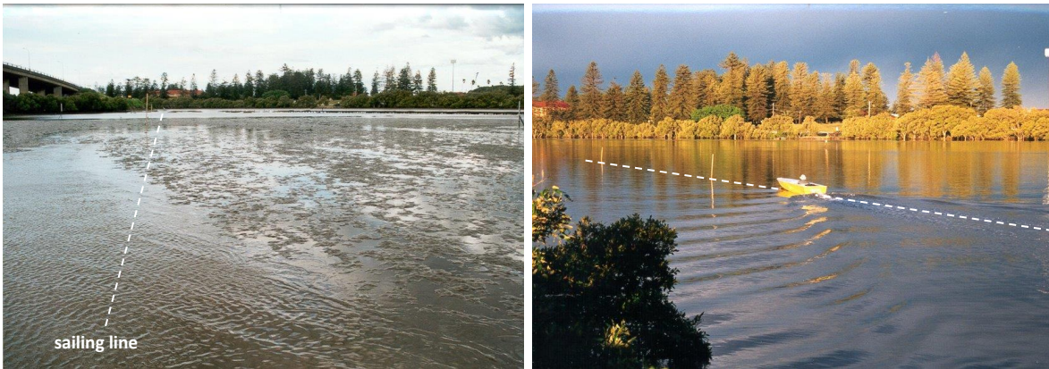
Figure 9.1 – Tests of a 7.375 m (LOA) self-propelled 1:8 scale model in water of approximately constant depth (no beach) conducted on the Hunter River in 1999. Left: A location was selected that dried at low water, allowing the course giving the most consistent depths to be chosen (and hazards identified). That also varied the h/L ratio naturally over the course of the tidal cycle. As flat as the bottom was, moderate depth variability at scale is acknowledged. Right: Testing in shallow water down to as little as 0.3 m depth ( h/L \sim 0.05 ), which was only possible with waterjet propulsion.
