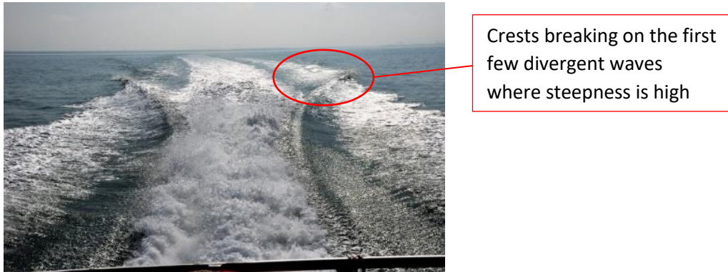
Figure 8.15 – Vessel travelling at Fr_L \sim 1.0 in deep water ( h \geq L ). The first divergent waves are steep, and their crests break periodically close to the sailing line. Breaking can also occur due to near-field interactions between bow and stern divergent packets. The near-field wake turbulence is caused by the water jet efflux.
