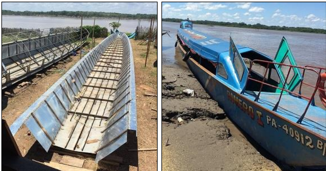
Figure 7.11 – An extreme example of a monohull river ferry (Rio Napo, Peru). The approximate dimensions are: L_{OA} = 33 m; B_{OA} = 2.6 m; B_{WL} = 2.0 m; \Delta = 10 - 12 t (laden), SR = \sim 13.5 . The service speed of 16 knots is achieved with three outboard motors of 170 kW total power. Passenger capacity is 70 persons. Construction is of thin galvanised steel sheeting with simple bench seating and canvas superstructure. Propulsion with outboard engines is not the most efficient at the service speed, but they are capital cost-effective, easy to service, simple to replace, and easy to refuel in remote locations. Photos courtesy of James Langner, Fibrecon Marine, Lima.
