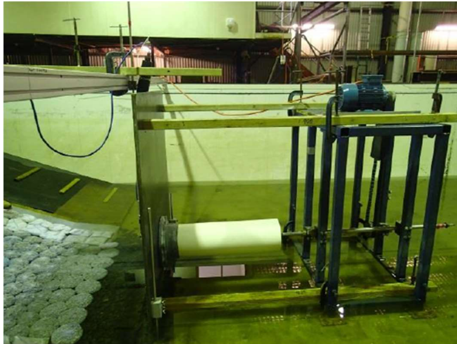
Figure 3 WRL basin showing bow thruster tube, motor (propeller inside tube) movable bed and Rock Bags
