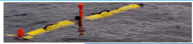
A 200 m depth rated AUV capable of being deployed from small vessel of opportunity and performing high resolution survey's. Features include Edgetech 2205B bathymetry and side scan system and Marine magnetics Magnetometer. Positioning can include an Applied Acoustics USBL Beacon correction giving high precision subsea positioning (HIPAP and GAPS Capable).
