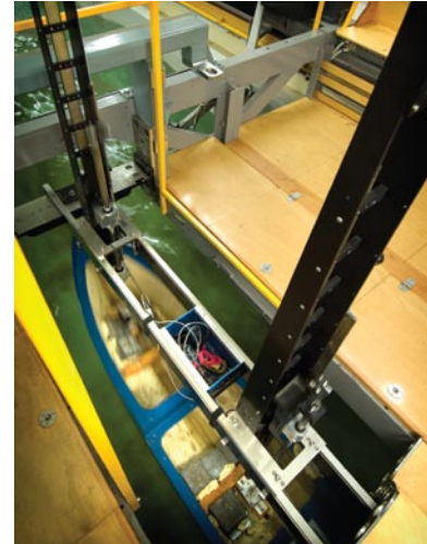
Model of AMC's training vessel Bluefin, ready for Towing Tank Tests
