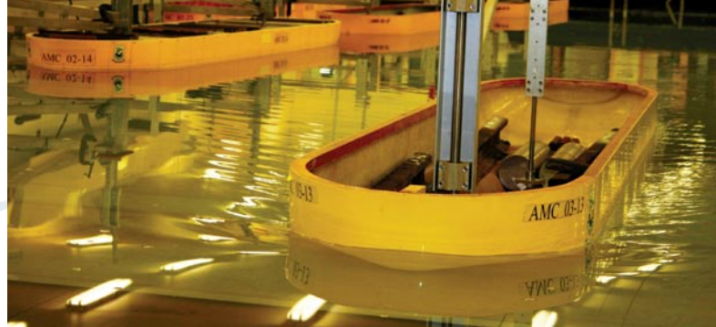
Vessel Interaction - Measurement of forces and moments on berthed bulk carriers by a passing ship
