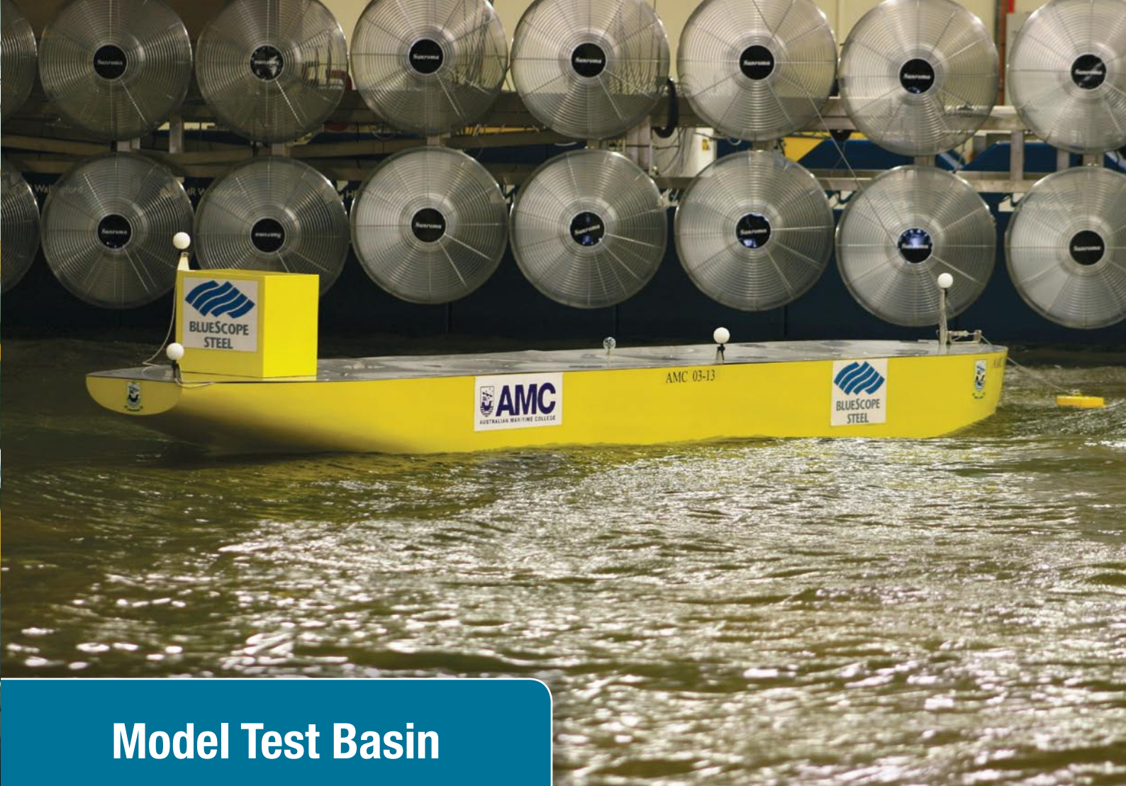
Measurement of six degrees of freedom motions in wind and waves (photo courtesy of BlueScope Steel)
