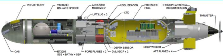
The Explorer class nupiri muka is a large modular AUV capable of operating in some of the most difficult conditions on earth, including beneath floating ice shelves. This vehicle has flexible payload options and can dive to 5000m and travel at speed between 1.0-2.0 m/s.
